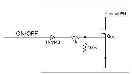
Fig1. Remote ON/OFF circuit inside power module
