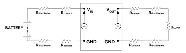
Test setup for efficiency
