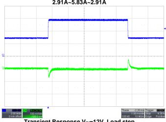
Transient Response V<sub>IN</sub>=12V, Load step 2.91A~5.83A~2.91A
