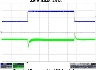
Transient Response V<sub>IN</sub>=10V, Load step 2.91A~5.83A~2.91A
