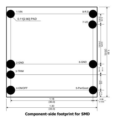
**Description PIN** 1  $V_{IN}$ 2 **GND** 3 TRIM 4 ON/OFF 5 **PwrGood** 6 **GND** 7  $V_{OUT}$ Remote Sense 8
