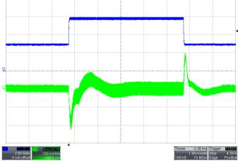
Transient Response V<sub>IN</sub>=6V, Load step 2.91A~5.83A~2.91A
