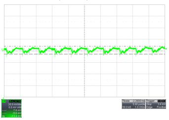
Noise V<sub>IN</sub>=12V, I<sub>O</sub>=5.83A, 5~20MHz Bandwidth
