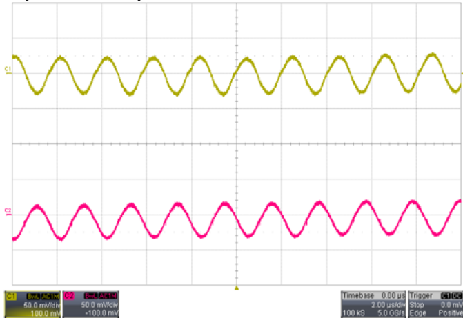
Ripple&Noise VIN=12V, IO=3A for both channel C1: Vo1; C2: Vo2
