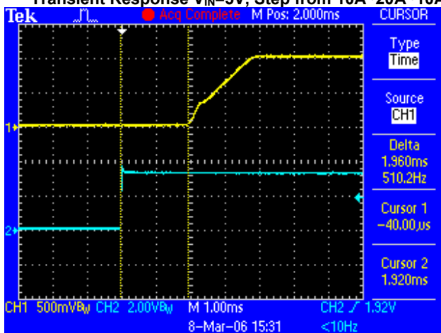
Start-up V_{IN}=3.3V , I_O=15.6A (resistive load)
