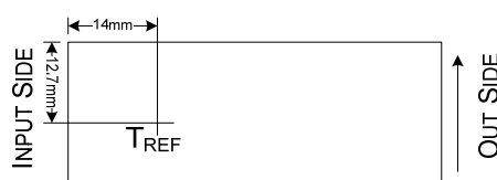
Fig 8 Case Temperature ( T_{REF} ) Measurement Location (Top view).
