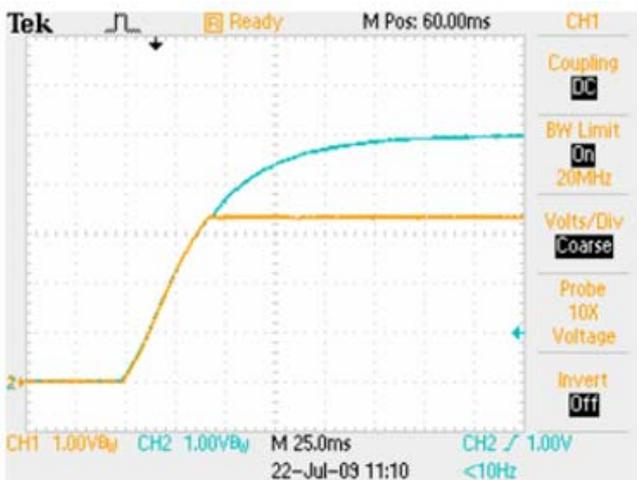
Power Up with *EasyTrack*<sup>TM</sup> Control  $V_{Track}=5.0V$ ,  $I_O=6A$
