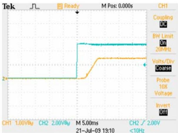
Start-up  $V_{IN}=5V$ ,  $I_O=6A$
