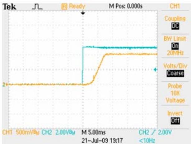
Start-up  $V_{IN}=5V$ ,  $I_O=6A$
