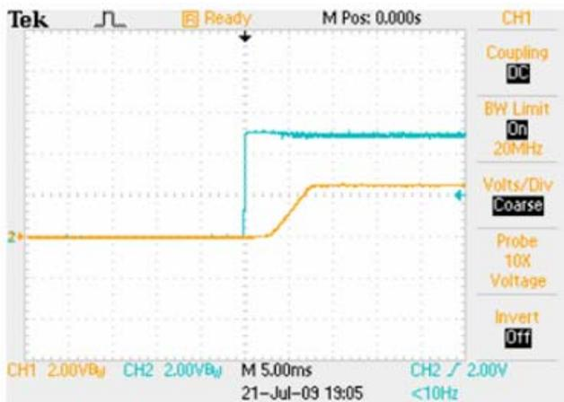
Start-up  $V_{IN}=5V$ ,  $I_O=6A$
