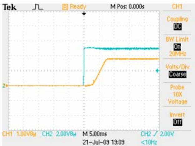
Start-up  $V_{IN}=5V$ ,  $I_O=6A$
