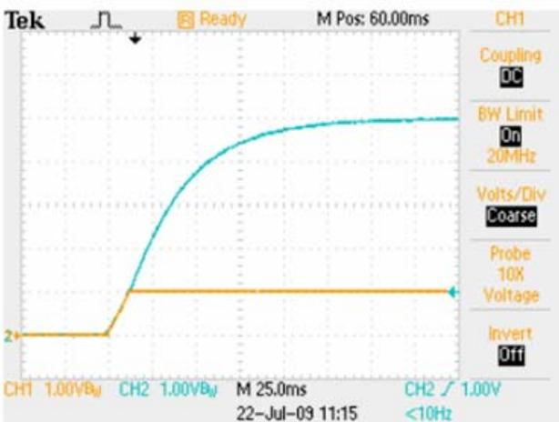
Power Up with *EasyTrack™* Control  $V_{Track}=5.0V$ ,  $I_O=6A$
