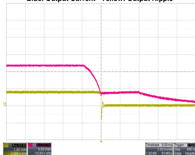
Shut-down V_{IN}=12V , I_O=100A Red: Input Voltage Yellow: Output Voltage
