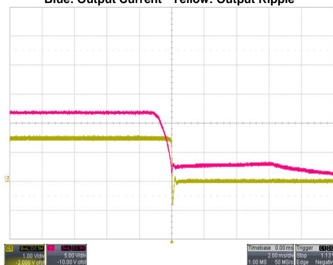
Shut-down V_{IN}=12V , I_O=50A Red: Input Voltage Yellow: Output Voltage
