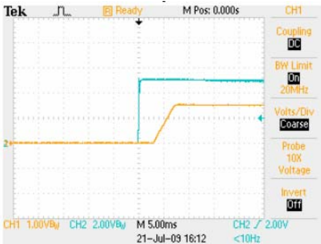
Start-up V_{IN}=5V , I_O=10A Yellow: Output Voltage Blue: Input Voltage
