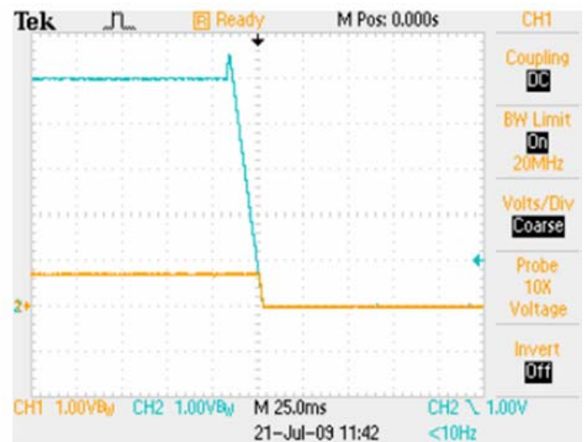
Power Down with EasyTrack™ Control V_{Track}=5V , I_O=10A Blue: EasyTrack™ Control Voltage Yellow: Output Voltage
