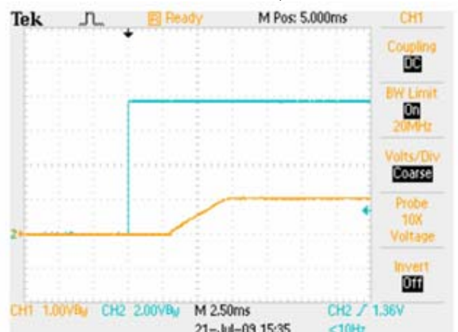
Power Up with ON/OFF Control, V_{IN}=11V
