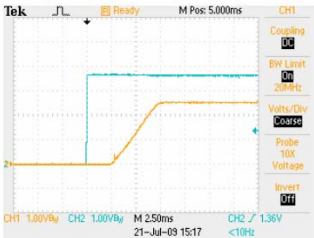
Power Up with ON/OFF Control, V_{IN}=5V Blue: ON/OFF Control Voltage Yellow: Output Voltage
