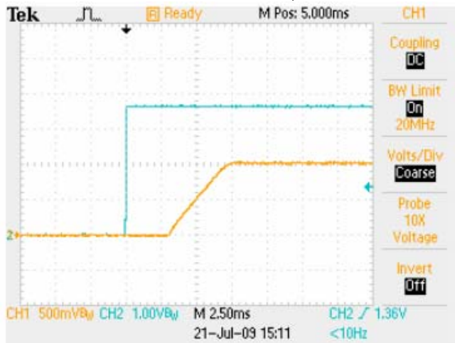
Power Up with ON/OFF Control, V_{IN}=5V
