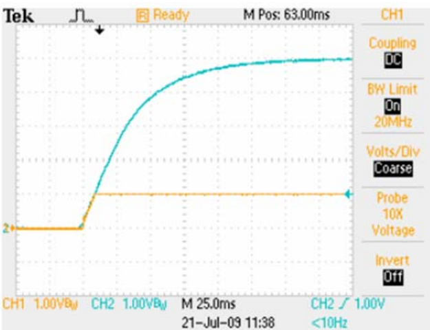
Power Up with EasyTrack™ Control V_{Track}=5.0V , I_O=10A Blue: EasyTrack™ Control Voltage Yellow: Output Voltage
