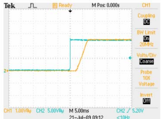
Start-up V_{IN}=12V , I_O=10A Yellow: Output Voltage Blue: Input Voltage
