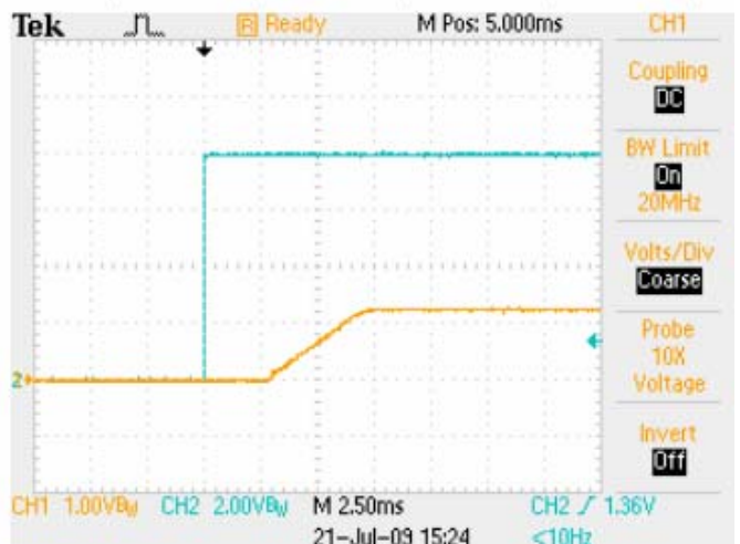
Power Up with ON/OFF Control, V_{IN}=12V Blue: ON/OFF Control Voltage Yellow: Output Voltage
