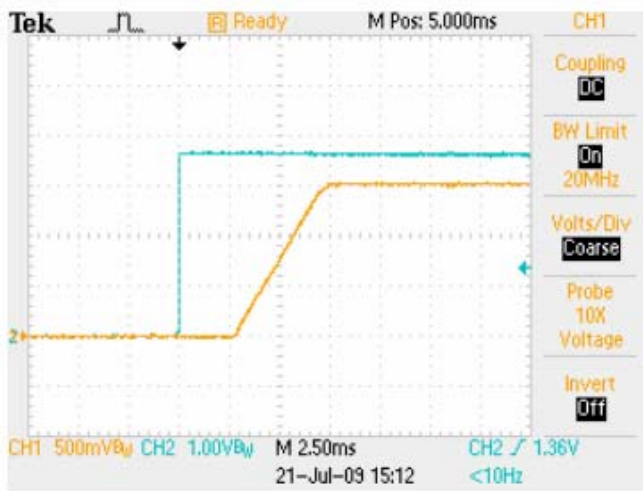
Power Up with ON/OFF Control, V_{IN}=5V Blue: ON/OFF Control Voltage Yellow: Output Voltage
