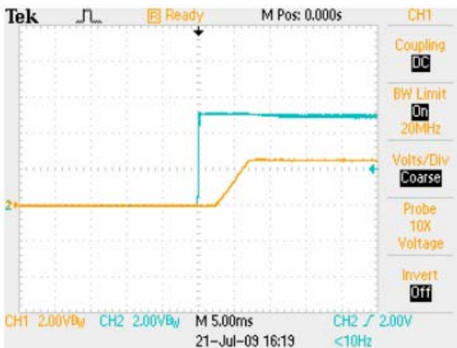
Start-up V_{IN}=5V , I_O=10A Yellow: Output Voltage Blue: Input Voltage
