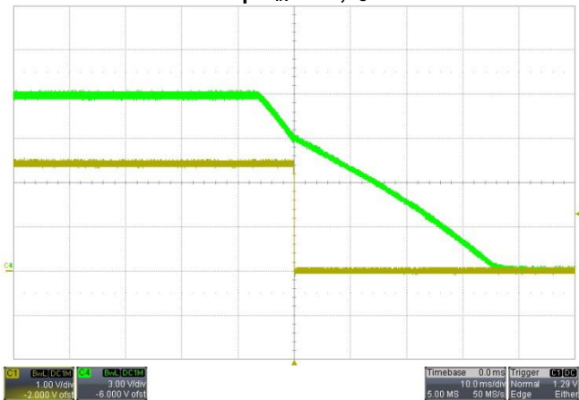
Start-up* V_{IN}=12V , I_O=6A Output filter 90*22μF Ceramic + 100μF TAN (150mΩ ESR)
