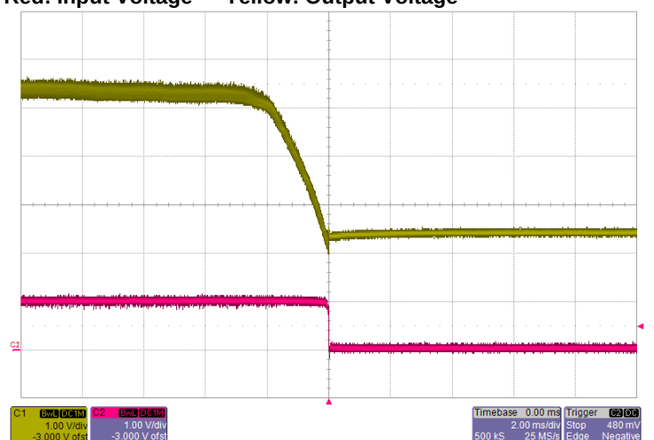
Shut-down V_{IN}=5.5V , I_O=10A Red: Input Voltage Yellow: Output Voltage
