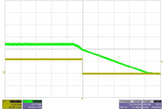
Shutdown V_{IN}=48V Green: Input Voltage Yellow: Output Voltage
